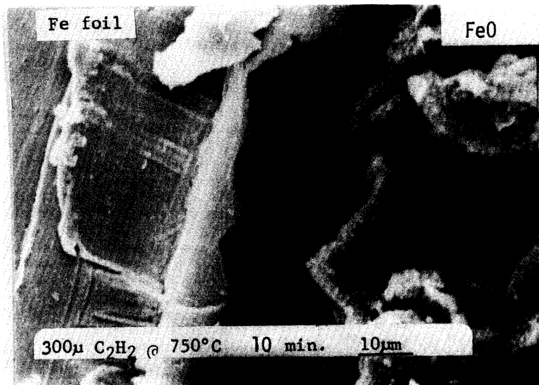
FIG. 5. The same region as shown in Fig. 4, after heating at 750°C in 0.3 Torr acetylene for 10 min.
