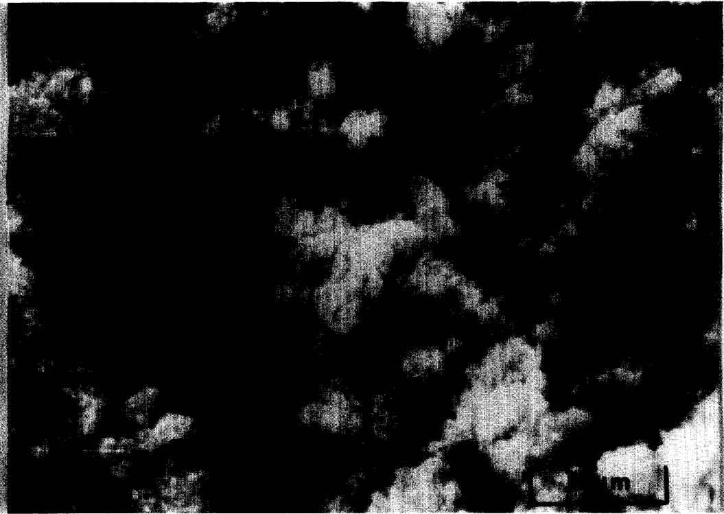
FIG. 3. The appearance of the same area of FeO shown in Fig. 2. After treatment in 0.3 Torr acetylene for 2 hr at 750°C.
