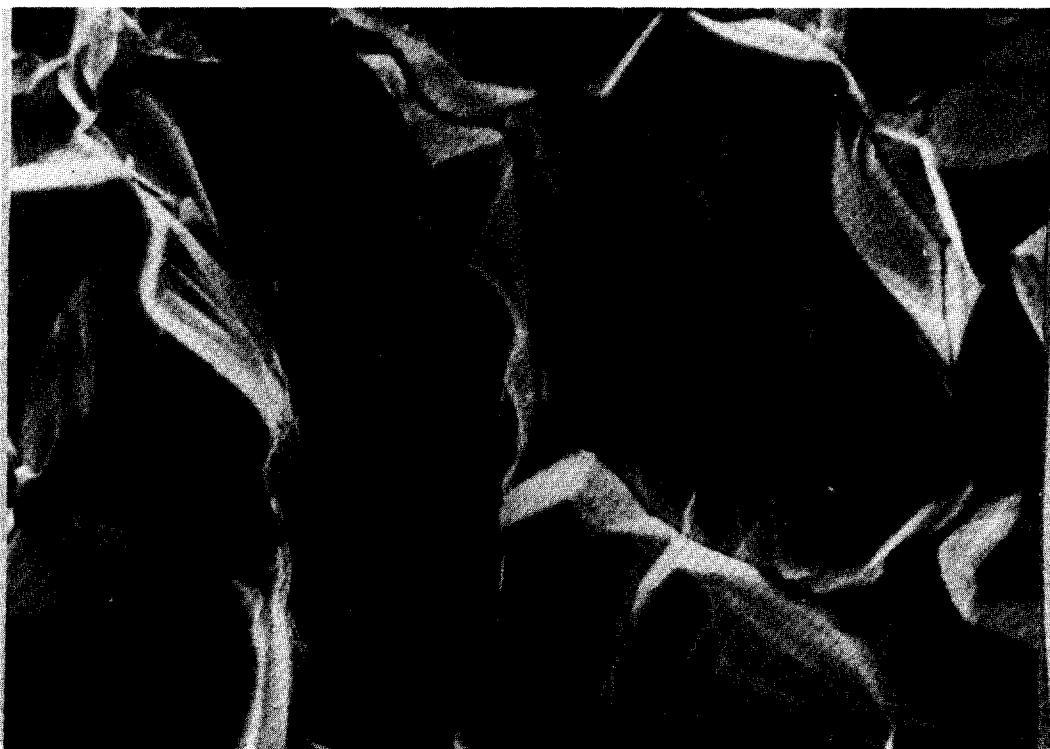
FIG. 2. Scanning electron micrograph of the surface of an FeO specimen.
